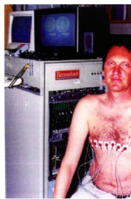
ACT3 imaging blood as it leaves the heart (blue) and fills the lungs (red) during systole. Thanks to D. Issacson.
