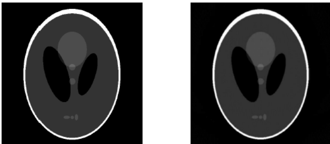
Reconstruction of the Shepp-Logan phantom. Left: original. Right: reconstruction with the filtered backprojection algorithm in [32].
